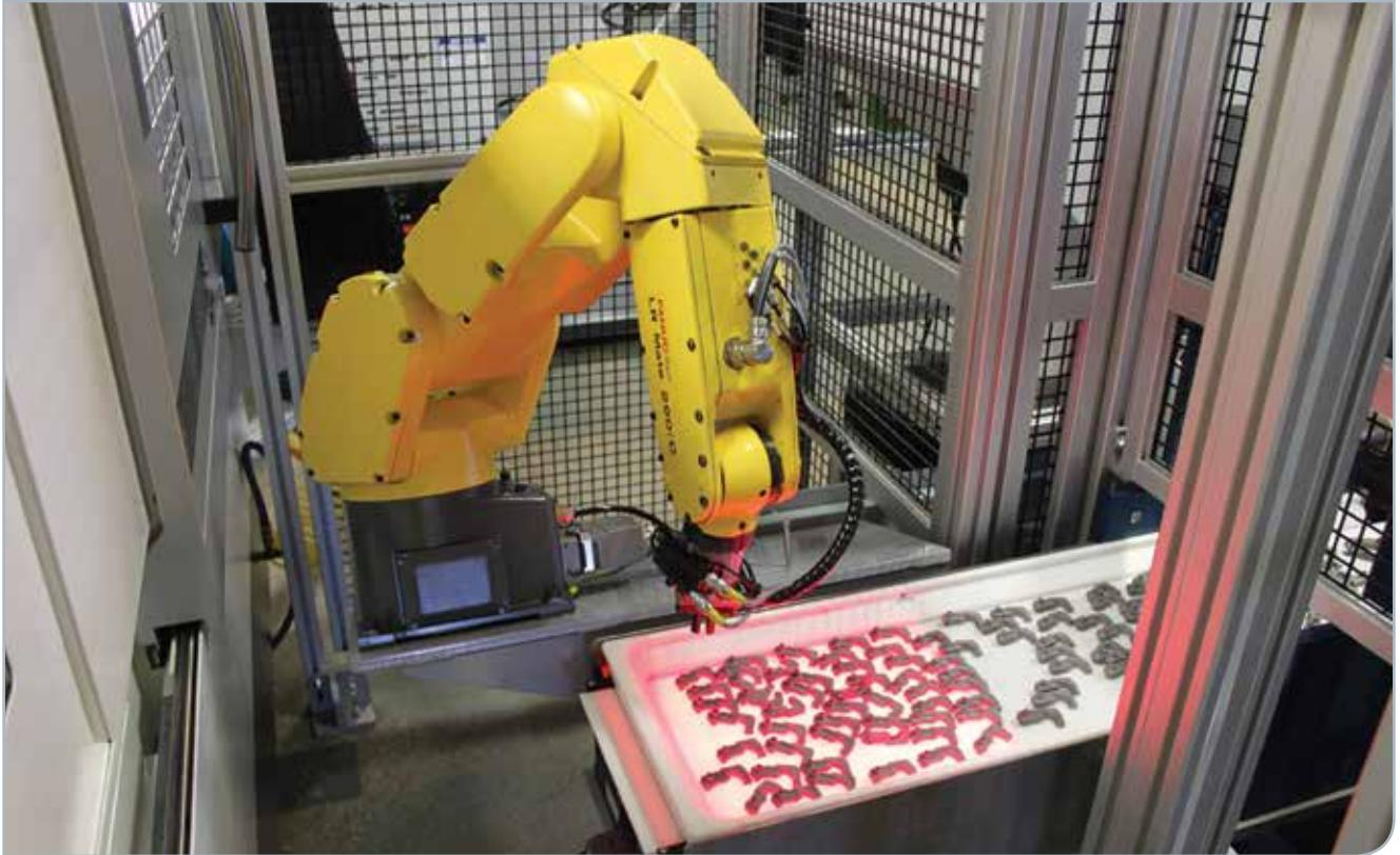
∴ The robot indexes the parts through the nests, loading a blank and unloading a finished part after each machine cycle, and depositing the finished parts onto a conveyor belt.
