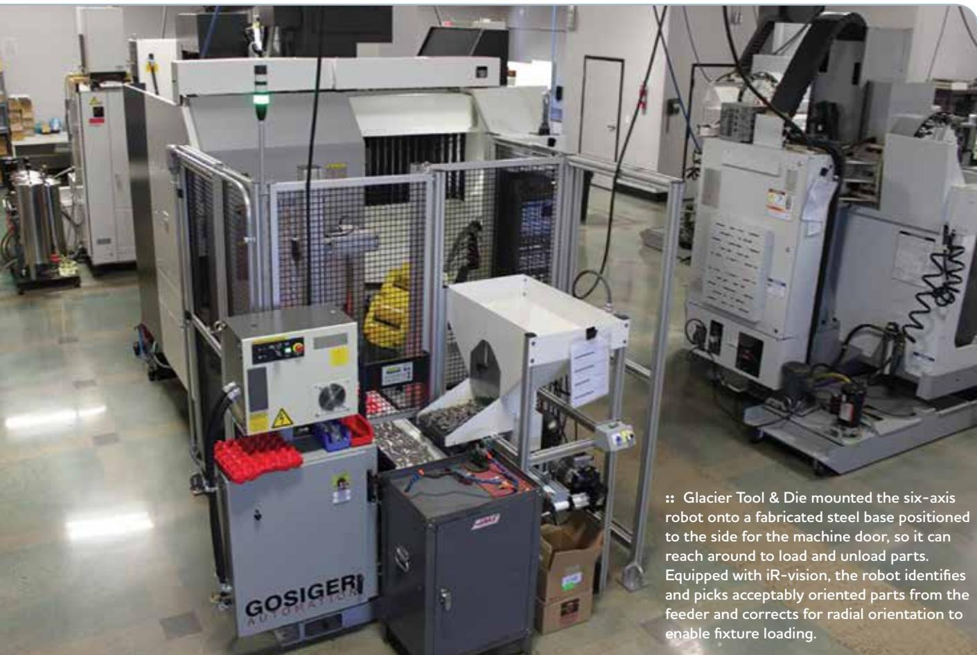
:: Glacier Tool & Die mounted the six-axis robot onto a fabricated steel base positioned to the side for the machine door, so it can reach around to load and unload parts. Equipped with iR-vision, the robot identifies and picks acceptably oriented parts from the feeder and corrects for radial orientation to enable fixture loading.
